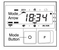
console will display the speed, time, distance, lap and calorie modes, for 5 seconds each, in a repeating cycle.
